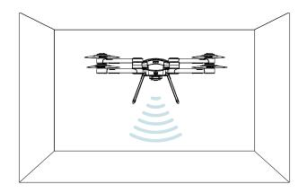
The precision of the visual and acoustic system can be affected by the illumination intensity and the surface texture of articles. And the ultrasonic will not measure the distance in certain damping materials. If both vision and ultrasonic do not work, the flight mode will be turned into the Attitude mode automatically. Therefore, please notice the following conditions during flight:
