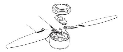
To remove, take down the propeller cap according to the direction shown in the cap. Lift the propeller cap up slightly and rotate it for  $90^{\circ}$  to remove the base. In the end, take down the propeller.
