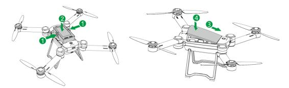
After flight, please take down the battery according to the method shown in the following picture. Take down the cover and press the snap joints at two sides of the battery at the same time. You can dismount the battery.
