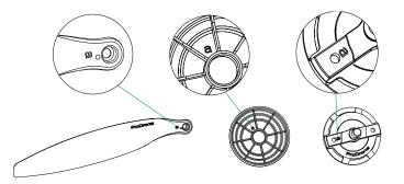
In installation, choose the same type of propeller with that on the motor rotor. Put the side with the letter up and insert it to the spacer pin of the propeller in the electric motor. Press the base of the propeller to the card slot of the motor spindle in the direction vertical to the spacer pin. Rotate for  $90^{\circ}$  to align the hole sides at two ends with the spacer pin and press it in. In the end, rotate the propeller cap according to the direction shown in the cap.
