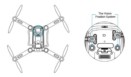
This system is adaptable to the environment in which the height is lower than 6 meters, where there is no GPS signal or the GPS signal is not good enough. It is particularly suitable for indoor flight.
