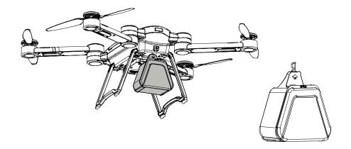
Before the ejection, the buttons C1 and C2 should be customized to choose the 'steering gear control' in the APP setting interface. The objects to be ejected are to be put into the container carrier and the container is inserted into the steering gear hole. Operate the aircraft to the place above the ejection point and press C1 or C2 button to let the container break away from the aircraft. The ejection is finished.
