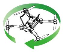
• Hold the aircraft with its **HEAD DOWN** and rotate it clock-wisely and vertically. Observe the color of the LED indicator light in the aircraft; the compass calibration is successful when the YELLOW lights at the head of the aircraft and the GREEN lights at the tail keep on. The compass calibration is not so good when all the yellow light keep on. You'd better calibrate the compass once more. Otherwise, please return to the step 2.
