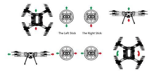
The default operation mode of the remote controller is the "American customization". You can modify with the parameter adjustment software or in "Control setting" on your APP. (See APP control setting for more details)
