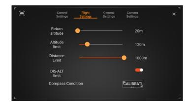
In this page, settings could be made for the Return Height, Altitude Limit, and Distance Limit. We strongly suggest you to set the altitude limit below 120m, although the maximum value allowed is 500m. If not, you will have to bear the risk.
