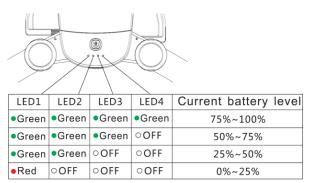
• After turning on the power switches of the aircraft and the remote controller, you could see the remaining capacity by observing the LED indicator lights for the aircraft in the remote controller.
