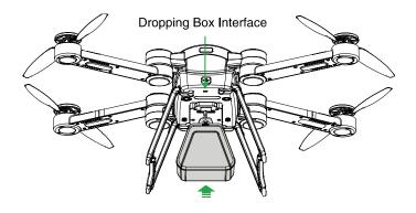
In dismounting, the powers of the aircraft and the remote controller should be turned on. And then the ejection would be carried out and the container would break away from the aircraft.
