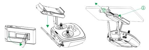
To remove, press down the 'Equipment support lock' and pull the support upward.
