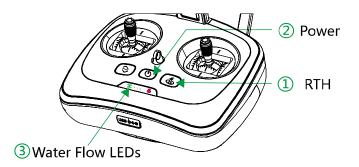
3. Press the power button of the aircraft for five times and wait for several seconds for the binding procedure to finish. At this time, the green LED indicator light showing the status of the remote controller is on.
