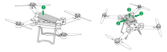
**%** Turn off the aircraft before taking out the battery.
