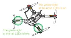
▲ Hold the aircraft head down and rotate it clock-wisely.
