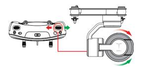
▲The camera button, video capture button and position reset button are all click buttons.
