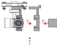
▲ Insert the Micro SD into the position shown on the gimbal.
