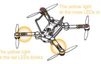
▲ Hold the ventral upward and rotate the aircraft clockwisely and horizontally.
