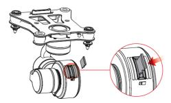
▲Turn off the power, and then insert the front snap joint into the mounted hole.
