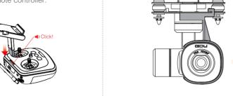
▲ Insert the Micro SD into the position shown on the gimbal.
